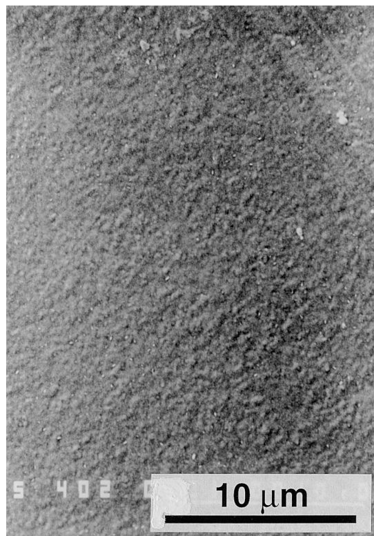
Figure 7. A surface SEM view of copoly(A-ProOEt/MA-Gly) (40/60 mol%) gel treated for 4 hr in a pH 3.0 buffer solution at 37°C.
